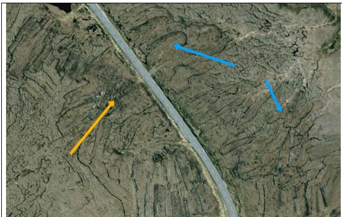
Figure 13. Aerial photograph of peat cuttings along the road running north from Stornoway, and identified as suitable locations for restoration proposals involving translocation of peat blocks from the development site to these cuttings. It can be seen that the majority of the cuttings are extremely well vegetated (blue arrows), with only small patches of bare peat (orange arrow).
