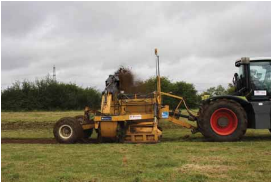
The rotary ditcher working at Rectory Farm near Buckingham © Mike Shurmer (RSPB)
