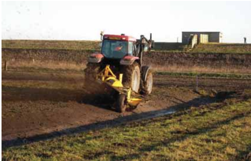
The BOS spoil spreader working on peat soils at the Ouse Washes © Mike Shurmer (RSPB)
