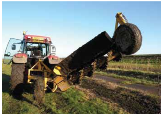
The BOS spoil spreader © Mike Shurmer (RSPB)
