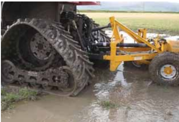
The BOS spoil spreader and SoucyTrack on a wet peat site and a foot drain created with this set up © RC Baker Ltd.
