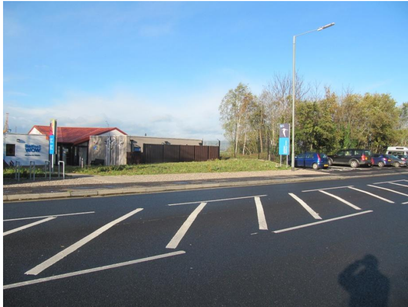
Figure 1 The path from the car park is tarmac and level, the path to the entrance is paved with a slight gradient
